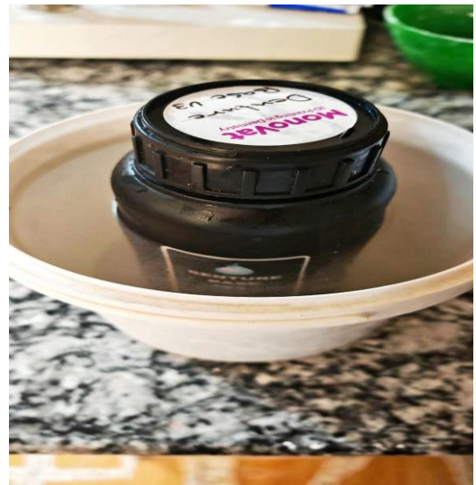
Figure 3: Resin Conditioning by Warm-Water Immersion Before Printing
